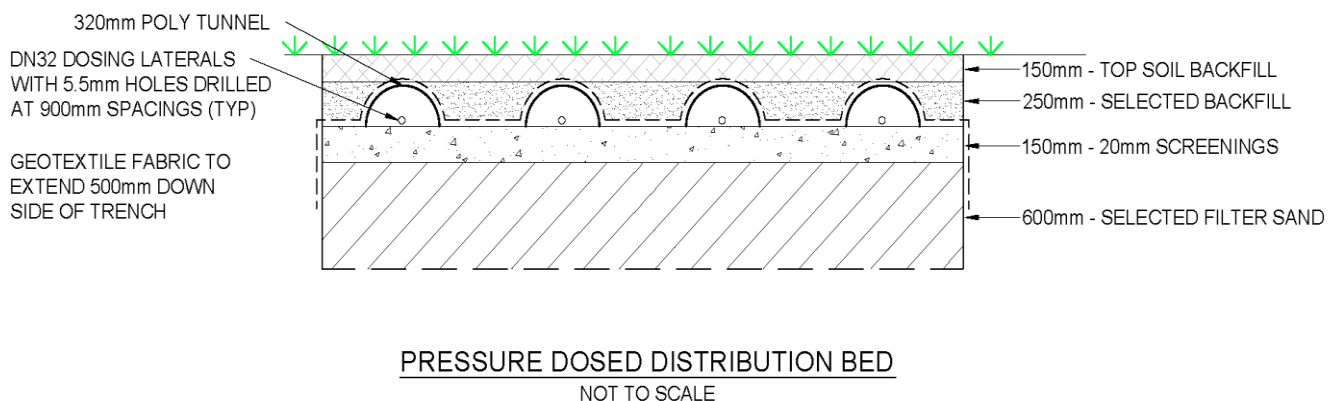
FIGURE 4-1 PRESSURE DOSED DISTRIBUTION BED (SOURCE: AWE – 2012)
