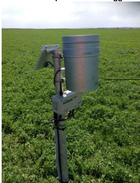
Plate 2 Solar powered data logger/controller with rain gauge
