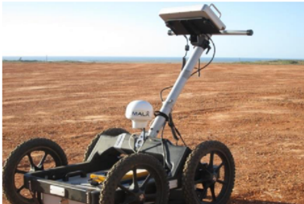
Figure 1: Example GPR cart setup
