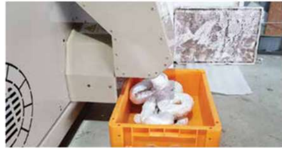
A polystyrene machine has been installed at the Waste Transfer Station which melts the product to be recycled into material for new products.
