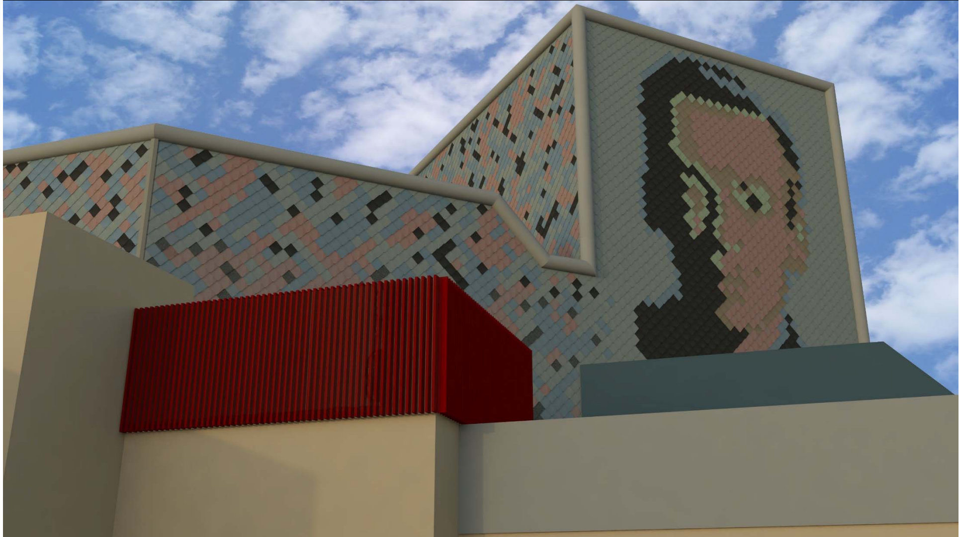
OPTION THREE - VMZINC ADEKA SHINGLE CLADDING, LOWER LEVEL ENHANCEMENTS & FLY TOWER 'PICTURE FRAME'
